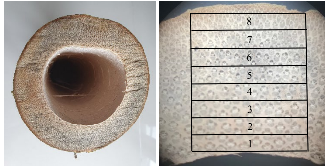
Fig. 3a. Cross-section area of internode bamboo b. A different layer of bamboo anatomy
